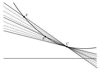
Figure 2.1. Sliding Secant Becomes a Tangent
